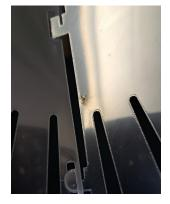
Place the middle tab in its slot, from the opposite side of the reflector.
