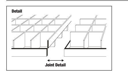
Interlocking step trim design permits panels to be butted together without a noticeable joint - providing an uninterrupted louver pattern. This jointing method is accomplished without having to reverse louver panels.
