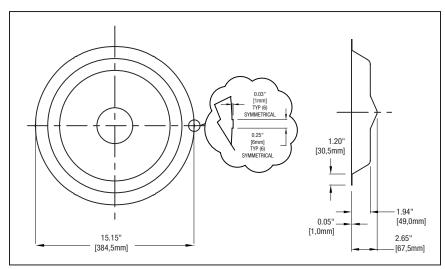
This drawing is for reference only. Actual part dimensions will vary. Customer is urged to review actual samples to confirm fit and function. All specifications and dimensions are subject to change without notice.
